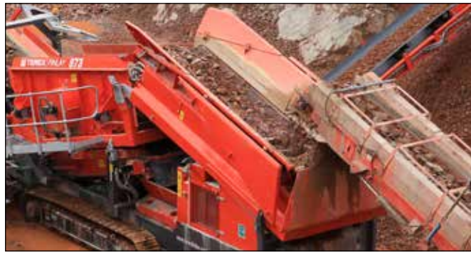
Hopper - Extensions folded for crusher feed
