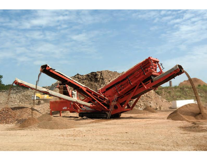
Building upon the highly advanced features of the QA440, the QA450 introduces a triple deck screen box and extra side conveyor that enable it to produce up to a total of four product materials.
