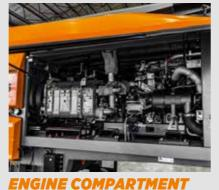
The engine compartment offers lots of space and easy access to all components, such as engine equipment, transfer case with direct engine connection or to the load-sensing system.
