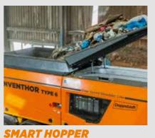
Extended feed area and automatic adjustment of material feed to increase the production of the shredding system.
