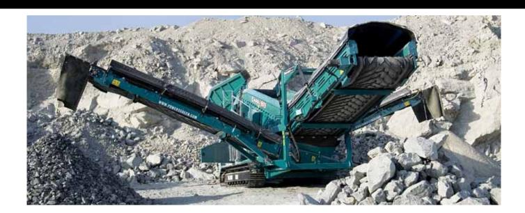
Designed for medium to large operators, where high capacity and throughput are paramount, the Powerscreen® Warrior 1800 is a tough, heavy duty machine built for screening, 2 or 3 way splitting and stockpiling in quarrying, recycling, construction and demolition aggregates and top soil applications.
