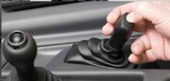
Body hoist lever with boost button
