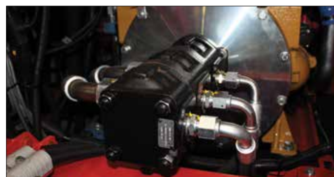
Pump 1: Triple 33cc/rev, 33cc/rev, 26cc/rev
