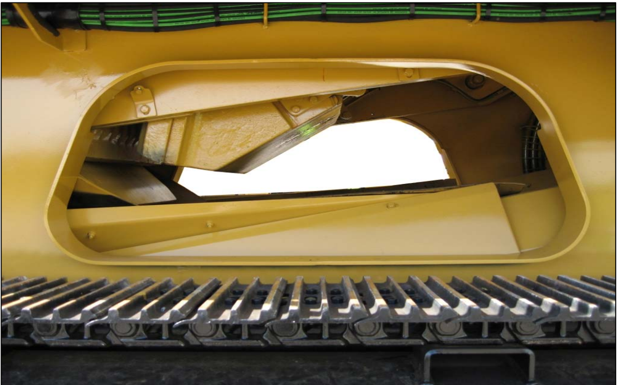
Large gap between discharge point of crusher and conveyor eliminates blockages and facilitates cleaning.
