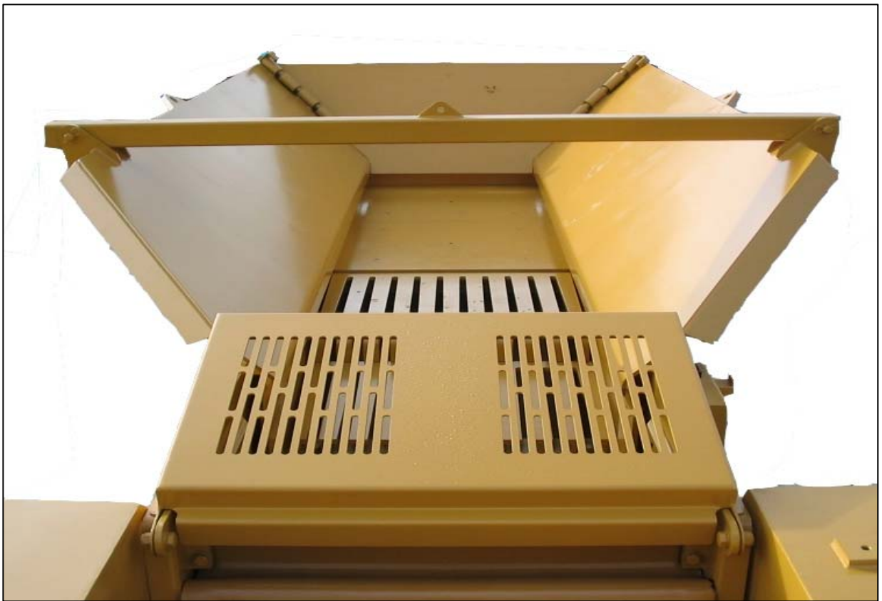
Large vibrating feeder with grizzly – flow of materials can be co-ordinated between the grizzly and jaw
