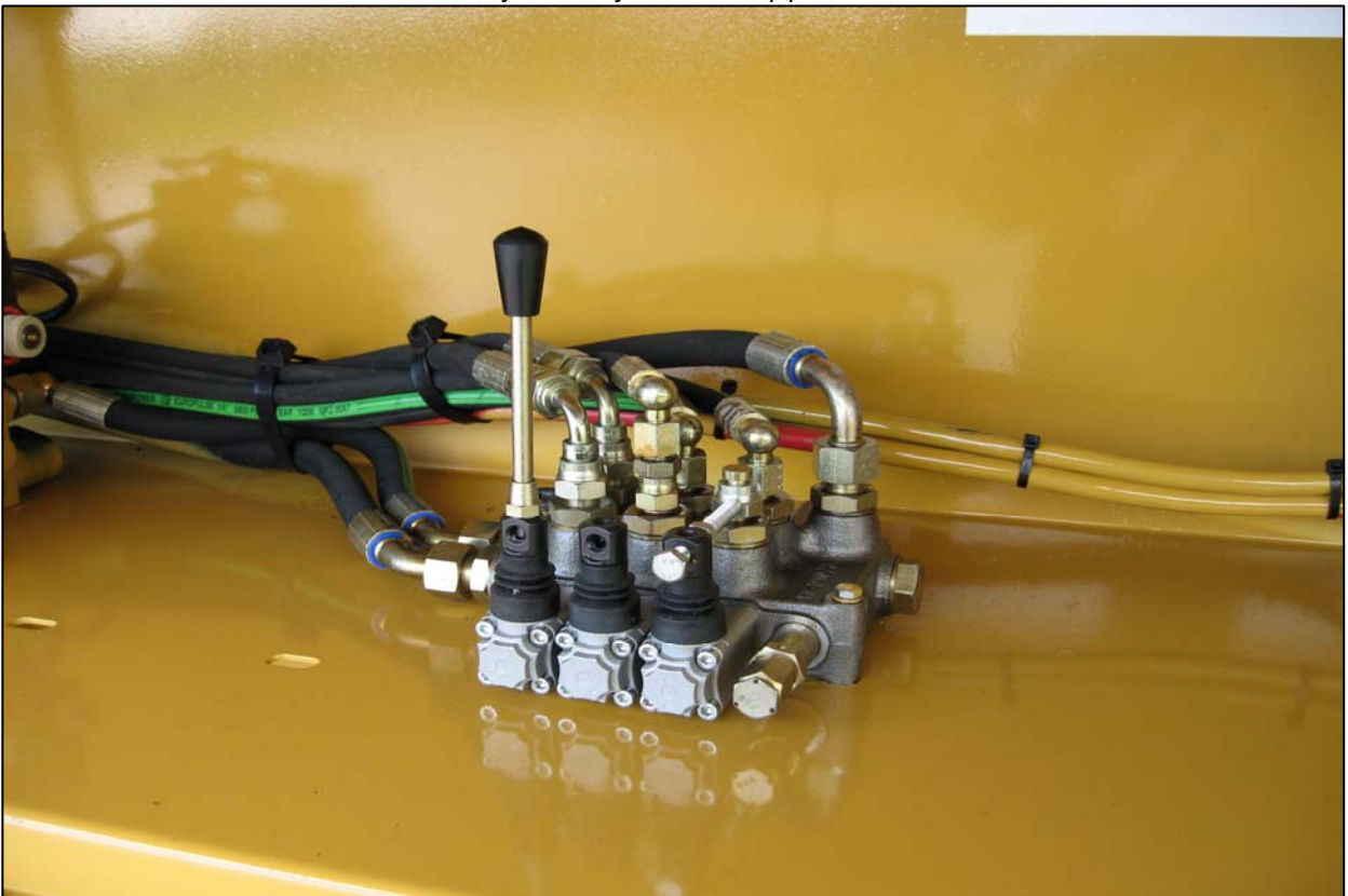
Extended main conveyor control
