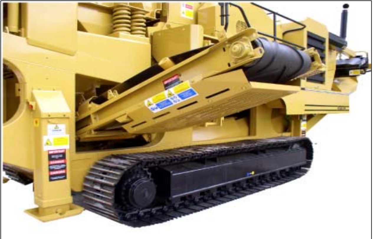
Side conveyor- collects fines passing through grizzly bars.
