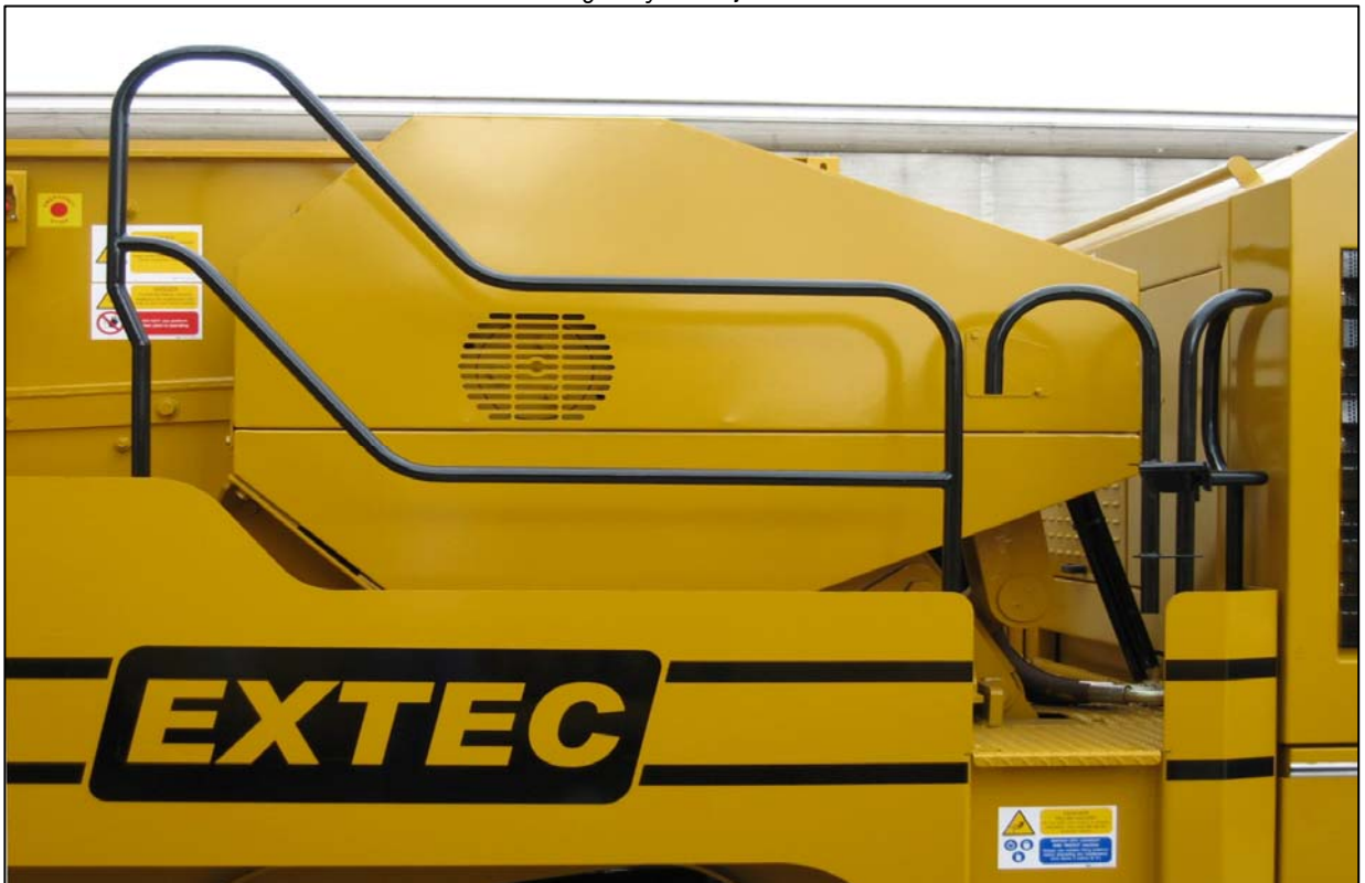
Maintenance platforms are provided on the right hand side of the crusher
