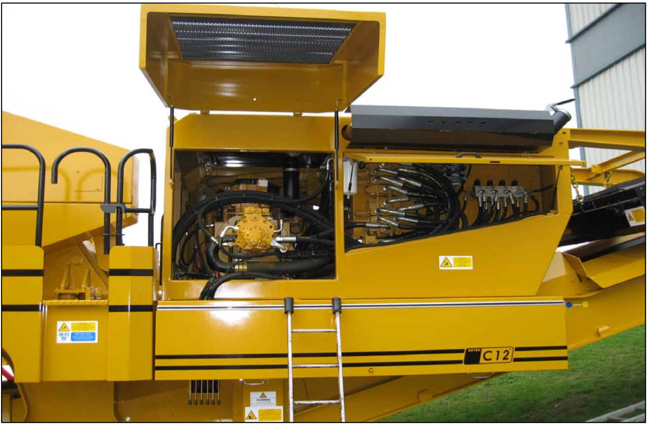
Caterpillar C-9 Powerpack- easy access for maintenance and service
