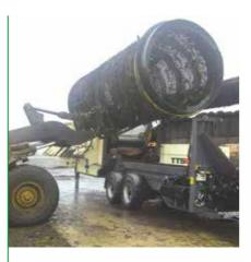
Easily replaced 5.5m (18') x 2m (6'7") punch plate drum which is compatible with the Doppstadt SM620 and Neuenhauser 6020
