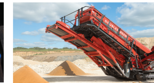
Three sided walkway around main conveyor
