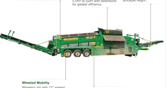
Wheeled unit with 72" spread tandem axle or tri-axle (REG).
