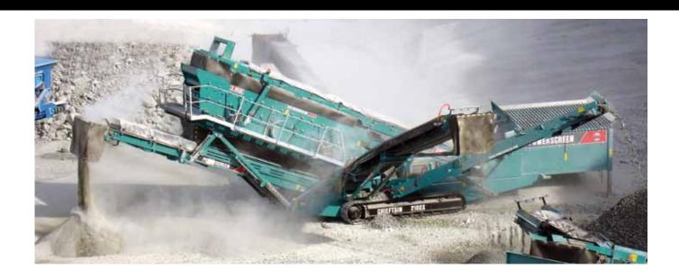
The Powerscreen® Chieftain 2100X is designed for medium to large scale operators who require large volumes of high specification products. The Chieftain 2100X is the largest model to feature a high capacity hopper, belt feeder and radio controlled tipping grid.
