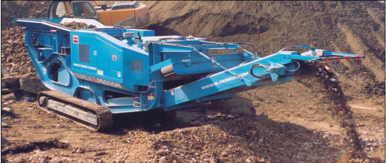
Above image features a Metrotrak fitted with the optional side conveyor and overband magnetic separator
